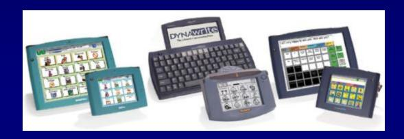
AAC devices provide communication access through typed or preprogrammed words and sentences, or through pictorial symbols.
